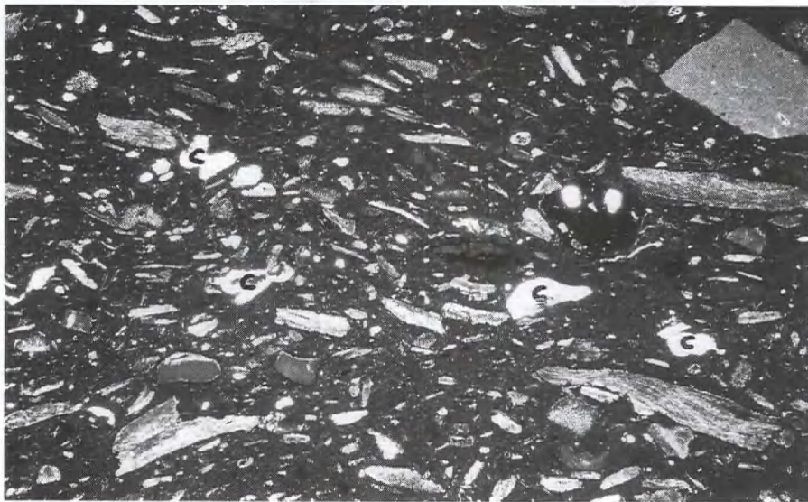
Plate 14. Photomicrograph of Pottery Sample 11. x20, XPL. C denotes calcitic inclusions.
